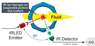
Figure 1 – Simplified arrangement for an IRLED-based turbidity instrument
